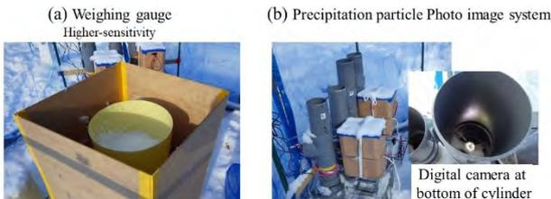
Fig. 2 (a) Weighing gauge with higher-sensitivity; (b) Precipitation particle imaging system.
