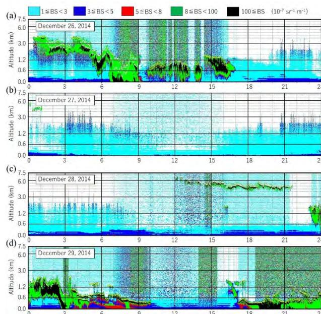
Fig. 9 Altitude-time cross-section of backscatter coefficient measured by the ceilometer from December 24 to 29, 2014.
