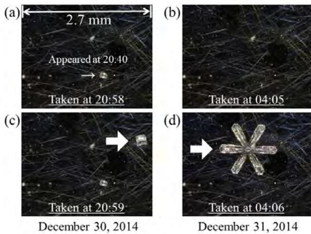
Fig. 6 Sequential precipitation particle photographs taken during EWP-II. Photographs captured at (a) 20:58 (JST) and (c) 20:59 on December 30, 2024, and at (b) 04:05 and (d) 04:06 on December 31, 2024. Bold arrows indicate particles that appeared within the 1-minute interval. The smaller arrow indicates a particle that appeared previously, with the corresponding time. The horizontal width of each photograph is 2.7 mm.
