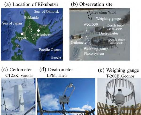
Fig. 1 (a) Map of Hokkaido showing Rikubetsu and topography of the region; (b) Landscape surrounding the observation site; (c) Ceilometer; (d) Disdrometer in the double fence windshield; and (e) Weighing gauge in the double fence windshield.
