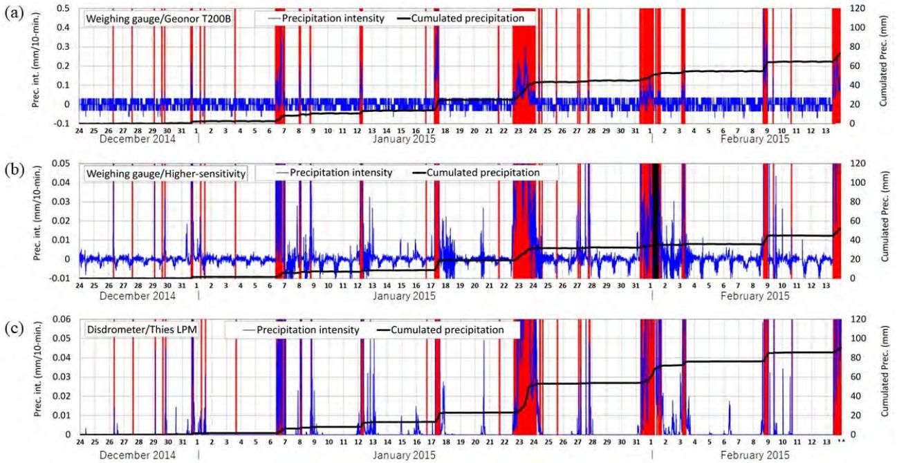
Fig. 3 Time series of precipitation intensity (mm/10 min) and cumulative precipitation (mm) from December 24, 2014 to February 13, 2015 for (a) the Geonor weighing gauge, (b) the higher-sensitivity weighing gauge (with approximately eight hours of data missing on February 1, indicated by black shading), and (c) the disdrometer. Periods when the Geonor weighing gauge detected precipitation exceeding 0.05 mm in 10 minutes are indicated by red shading.
