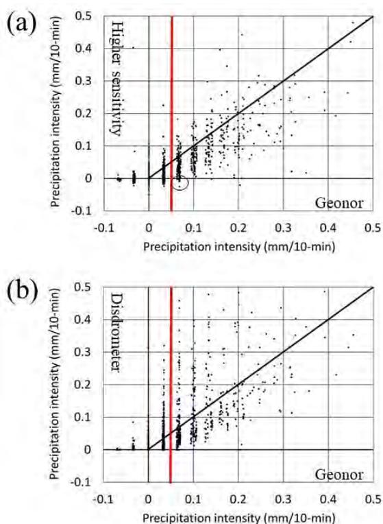
Fig. 4 Comparison of measured precipitation intensity between instruments. (a) Geonor weighing gauge vs. higher-sensitivity weighing gauge; (b) Geonor weighing gauge vs. disdrometer. Precipitation events detected by the Geonor weighing gauge are plotted to the right of the red vertical line (0.05 mm/10 min). The circle in (a) indicates the reference area discussed in the text.
