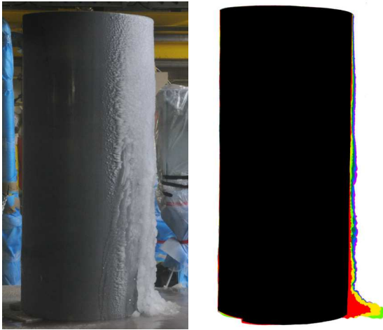
Fig.6 Cross-section area of the spray ice. Left: a PVC cylinder of 520mm diameter (#MV520), Right: difference between the trimming area including the spray ice and the projected area of specimen.
