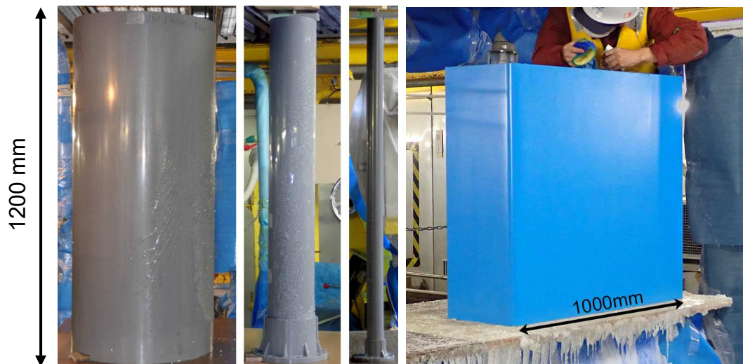
Fig. 2 Flat-plate and cylindrical specimens. Diameters of cylindrical specimens (left) are 520 mm, 165 mm, or 60 mm.
