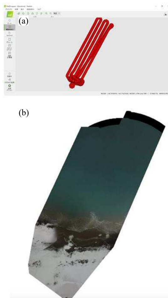
Fig 4. (a) Flight path of each aerial photo on Pix4D mapper software and (b) Orthomosaic rectified image.
